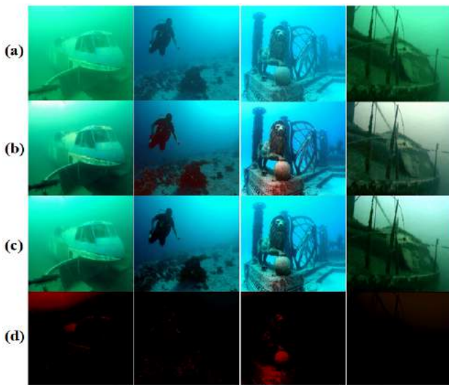
Fig. 13. Samples of the images presenting unbalance in color channels and outlier pixels treated by the attention module. (a) Input image; (b) Output image; (c) Output image with the attention module inserted in degradation function; (d) Image from the attention module algorithm.
